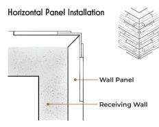
**Option 1:** A seamless outside corner can be achieved by joining panels using a miter joint.
